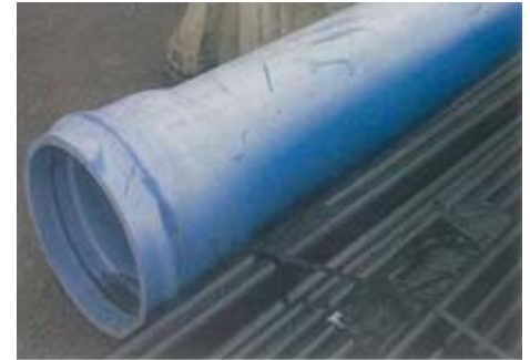
Figure 1: Surface discoloration of PVC pressure pipe stored outdoors, unprotected for 15 years. The discolored pipe passed all test requirements for new pipe.
