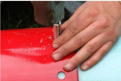
Step 4 – Install the slotted roll pin into the pin hole. The roll pin should extend through both pull head and the PVC pipe.
