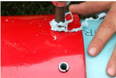
Step 5 – After installing the first roll pin continue to install all the remaining roll pins.
