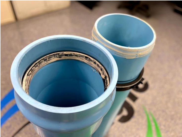
Figure 5: Example of lubrication to the gasket and the bevel only.
