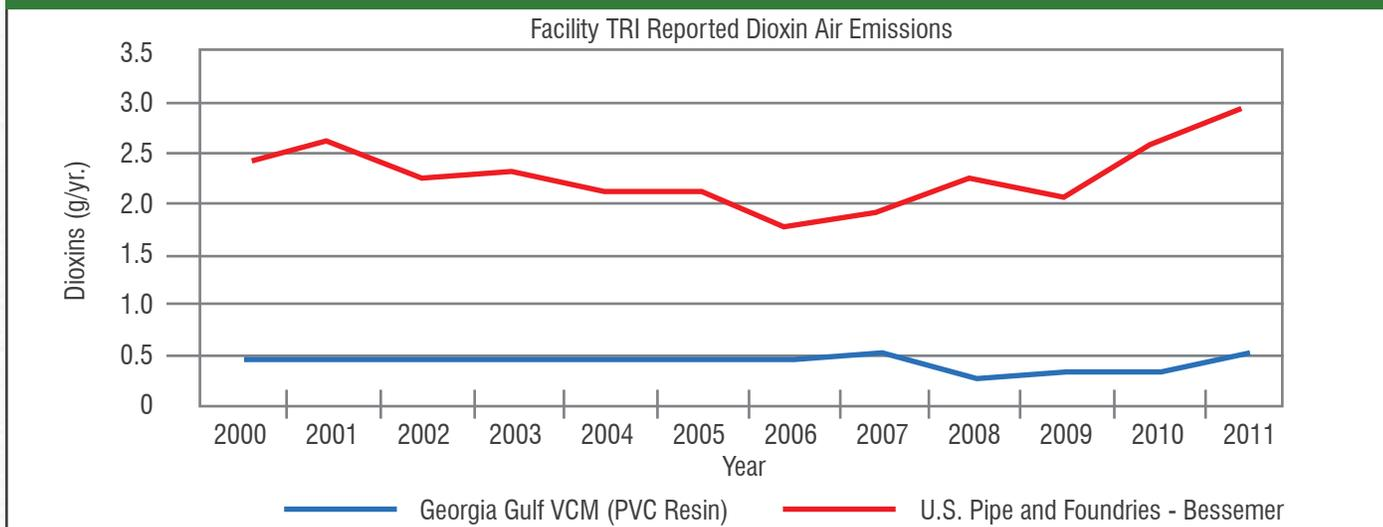
Dioxin emissions are tracked by the U.S. EPA through the Toxic Release Inventory (TRI). TRI data are made publicly available. Figure 5.2 is a sampling of the dioxin air emissions reported by a VCM (PVC resin) manufacturer and a ductile iron manufacturer.<sup>35</sup>
