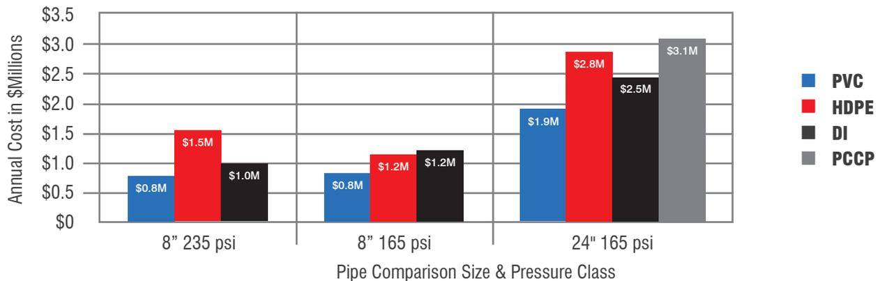
The average annual pumping cost savings for 8-inch pipe using PVC instead of DI can be up to \$440,000, and the savings using PVC instead of HDPE can be up to \$770,000.
