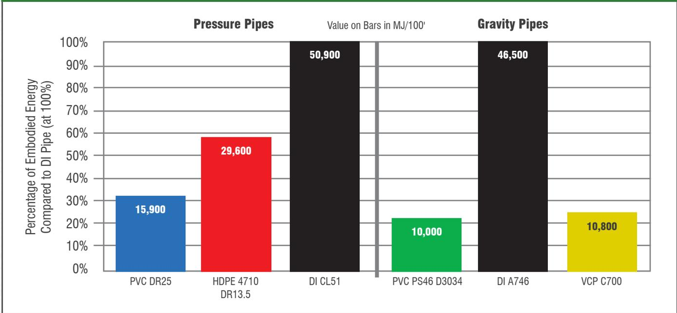
Note: Total 100-year embodied energy includes cradle-through-installation, required replacements and corrosion protection.
