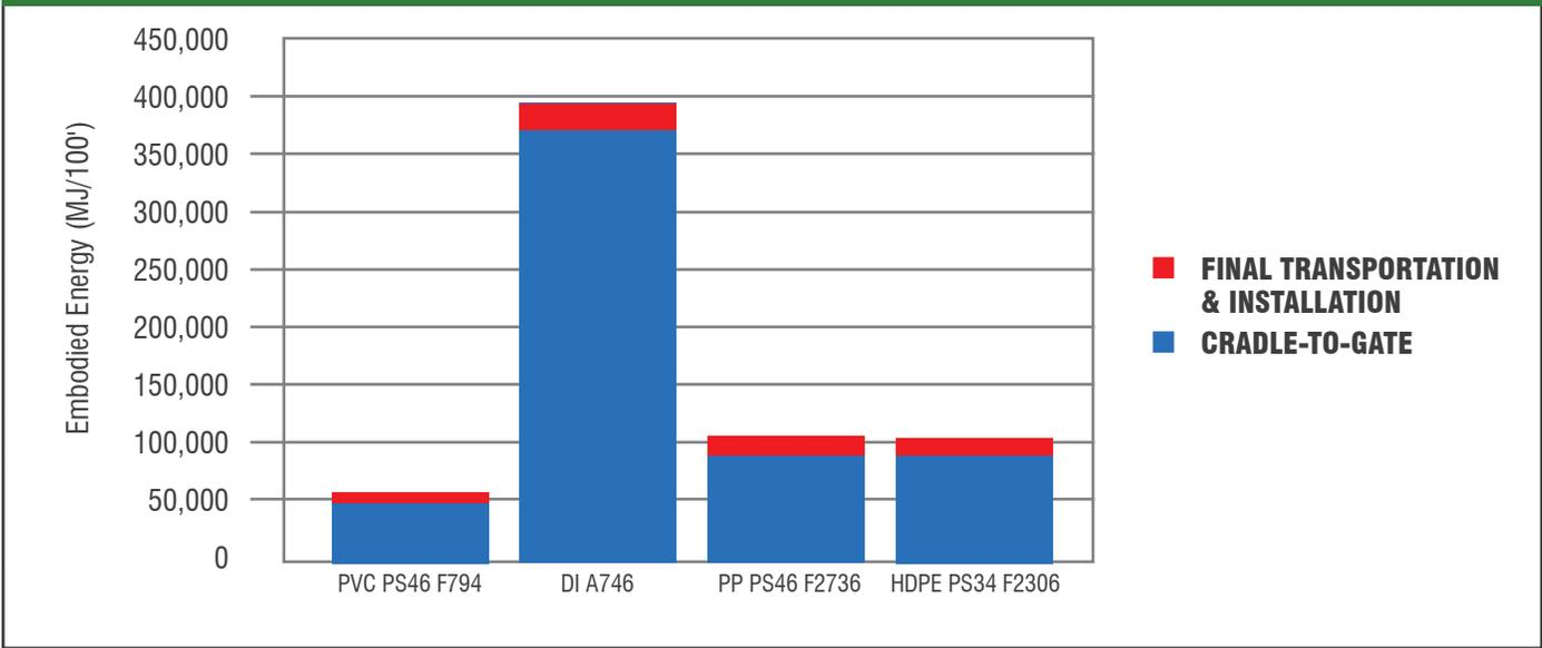
Figure 12.7 compares 24-inch PVC profile-wall, DI, PP and HDPE pipes equivalent to PVC PS46 F794 profile-wall pipe. The total 100-year embodied energy of PVC sewer pipe is 85 percent less than equivalent DI sewer pipe; 44 percent less than PP and 43 percent less than HDPE sewer pipes. It should be noted that the equivalent HDPE sewer pipe has a pipe stiffness that is 26 percent less than the pipe stiffness of PVC pipe.
