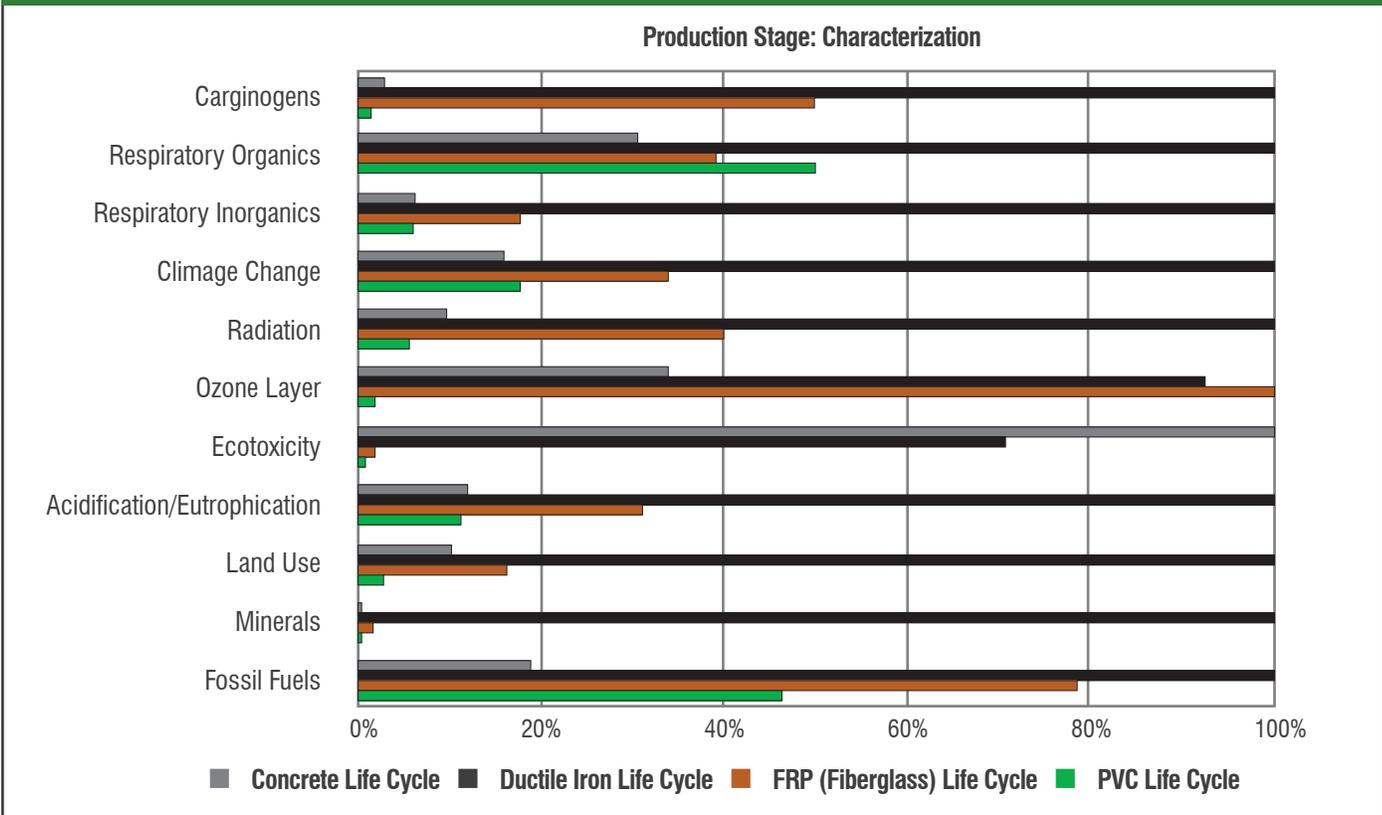
**FIGURE A.28 : SINGLE SCORE GRAPH FOR LIFE CYCLE COMPARISON FOR ALL PIPING MATERIALS**
