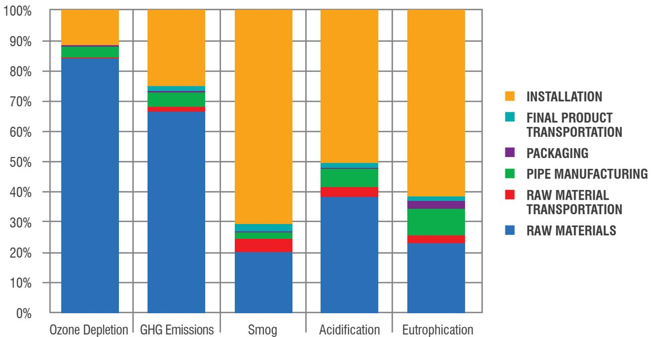
**TABLE 4.3 : 8” PVC DR25 PC165 C900 PRESSURE PIPE ENVIRONMENTAL IMPACTS USING THE TRACI IMPACT METHODOLOGY**
