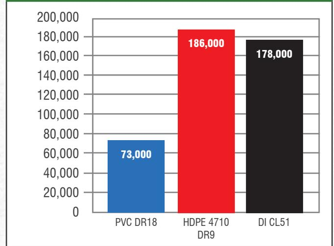
**FIGURE 10.4 : COMPARISON OF AVERAGE ANNUAL 100-YEAR PUMPING ENERGY COSTS PER 1,000 MILES OF PIPE BASED ON 0.4 FPS VELOCITY**
