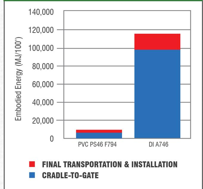
Figure 12.6 compares 8-inch PVC solid-wall, DI and VCP gravity pipe materials equivalent to PVC PS46 D3034 solid-wall pipe. The total 100-year embodied energy of PVC sewer pipe is 88 percent less than equivalent DI sewer pipe and 64 percent less than VCP pipe.
