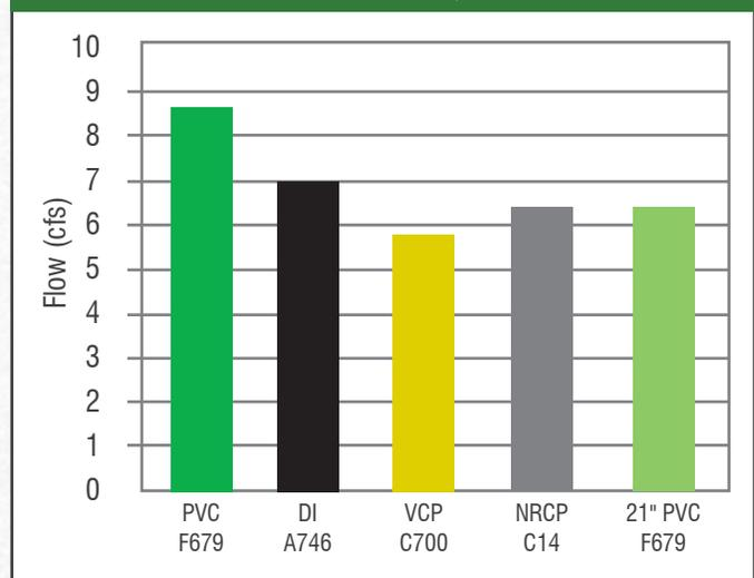
Figure A.13 compares PVC ASTM F679 pipe to other 24-inch solid-wall products. PVC has over 24% more capacity than DI pipe, over 50% more than clay pipe, and 35% more than non-reinforced concrete pipe (NRCP) on the same slope.
