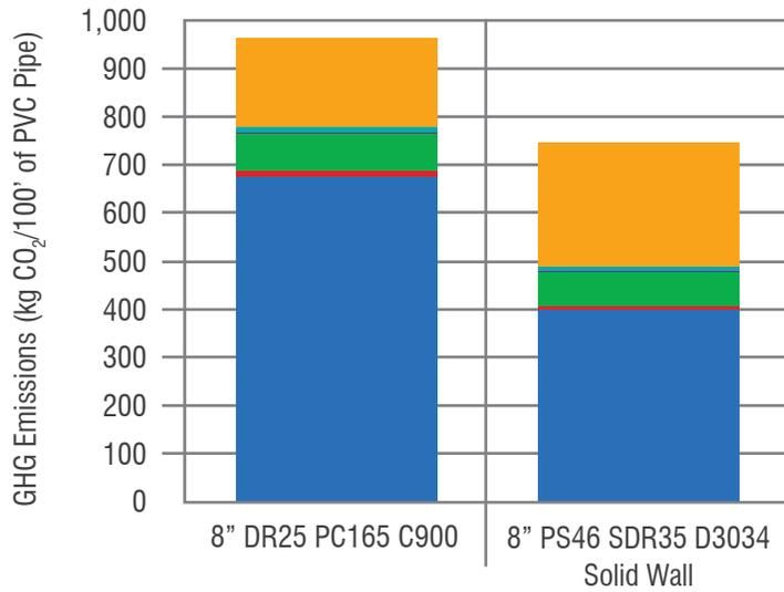
For these two piping products, the raw materials stage is the main driver of impacts; however, the installation stage is also a large driver of GHG emissions.
