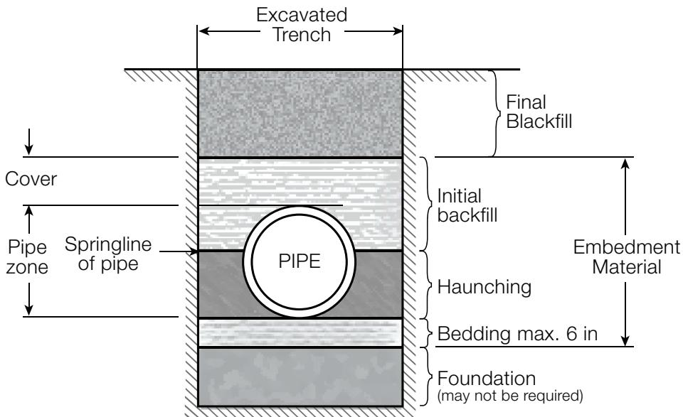
As shown in Figure 1, a PVC pipe trench is separated into several zones, each with a different function:
