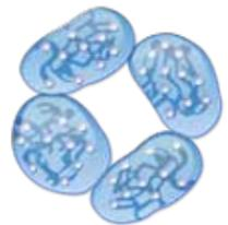
CONVENTIONAL PVC PIPE CLUSTERS THE MOLECULES, REQUIRING A THICKER WALL FOR STRENGTH.
