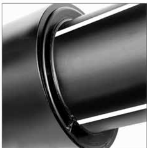
Figure D Correctly Made Socket Fusion Joint
